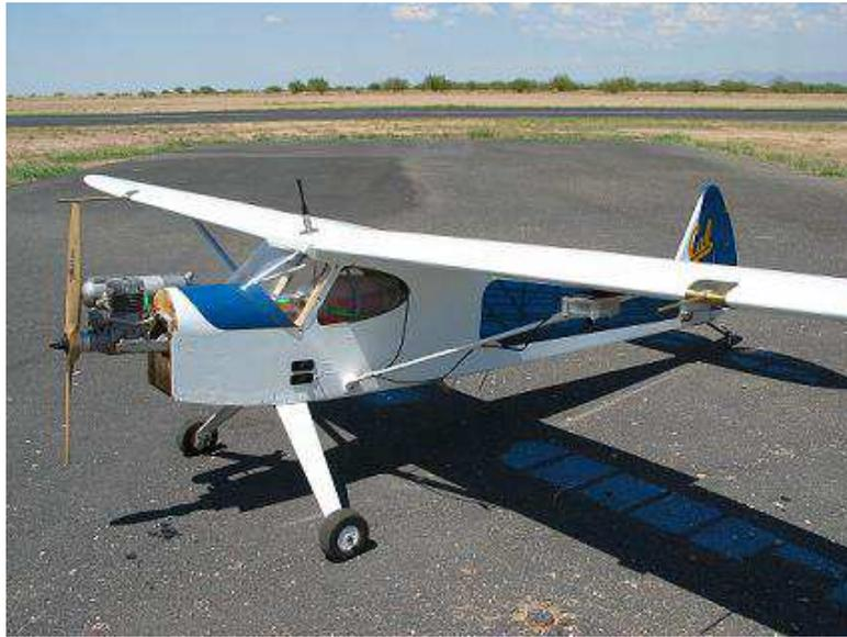
Figure 4. The modified Sig Rascal aircraft. Note wing-mounted bullet camera and payload access port above landing gear.
