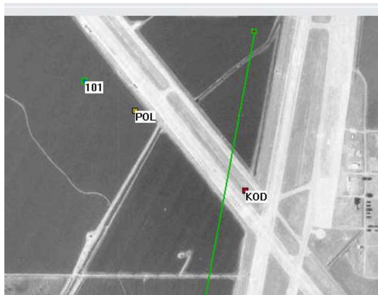
Figure 2. Part of the map area of the Team Control interface. The UAVs Polar and Kodiak are shown, as well as a visit task (101) and part of a border patrol task (diagonal line).
