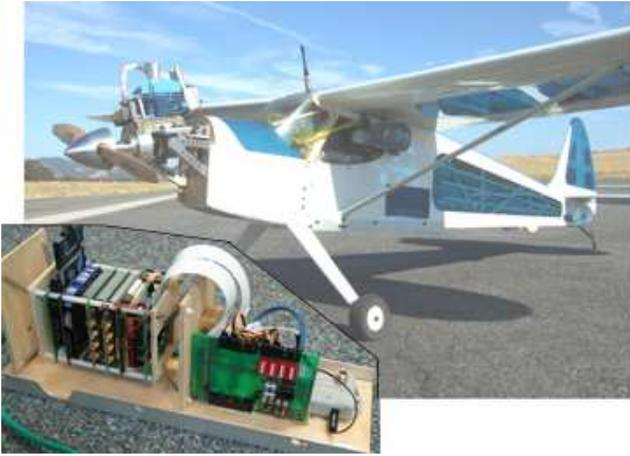
Fig. 1. Sig Rascal airframe and payload tray with vibration isolated PC104 computer
