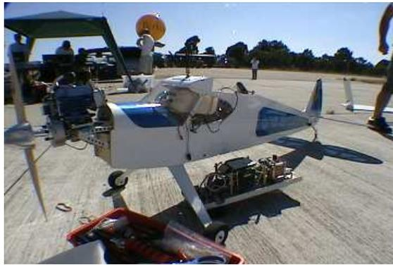
Fig. 2. Unmanned aerial vehicle.
