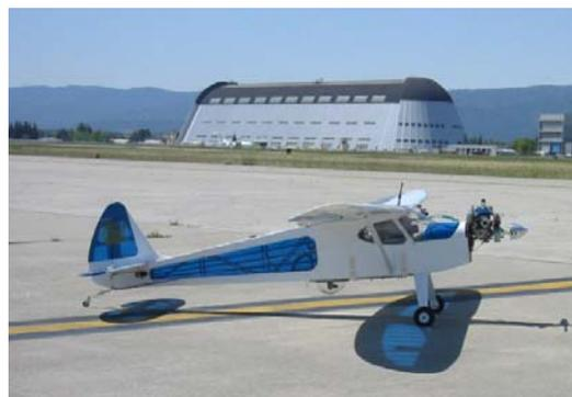
Fig. 1 UC Berkeley fixed wing UAV testbed.
