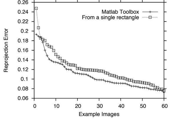
Figure 3: The vanishing point-based algorithm was compared with the *Calibration Toolbox for Matlab*<sup>®</sup>. The Toolbox used all  $5 \times 5$  points while the proposed approach only used the 4 corner points. For both of the methods, average reprojection errors of all  $5 \times 5$  points were calculated. The graph shows the sorted errors for all the examples. The Toolbox is slightly better but the difference is very small compared to the variations of the errors within a single method.
