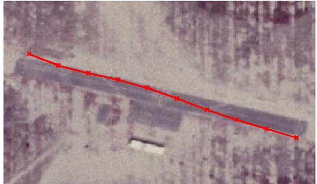
**Figure 14** - Results of road tracking on actual aircraft.
