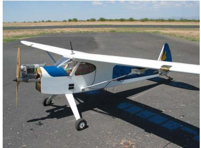
**Figure 1** – The experimental autonomous aircraft is a modified Sig Rascal radio-controlled airplane with 110 in. wingspan.
