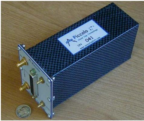
**Figure 8** - Cloud Cap Piccolo avionics package
